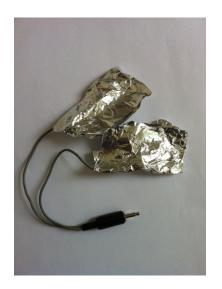
Connect the puppet to the **sensor board** using a **switch**, or connecting two wires with aluminum foil.
