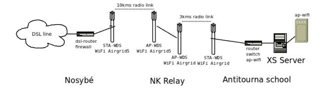
On the school, a normal Internet access architecture was configured with a switch connected to the receiving UBNT Airgrid5 and to the XS server as Internet Gateway for the local wireless network and the local services for the XOs. The XS has 2 network interfaces (one for Internet and one to the local wireless router in bridge mode to serve connectivity to the XOs)
